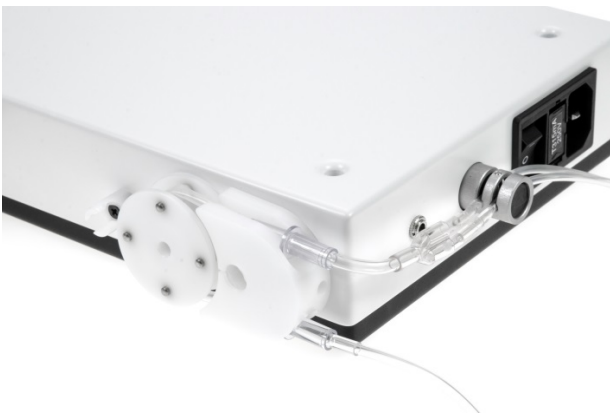
Figur 7 Anbring de to slanger i klemmeventilen
