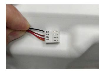
Connect the cable to connector J108 on the chair PCB.
