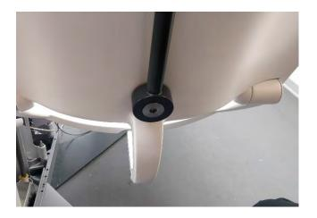
Adjust the friction of the suction holder with the hex nut and a hex key size 10. The friction should be equal to 1kg when using a dynamometer/fish weight.
