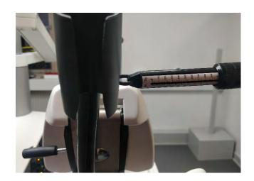
When the hex nut is adjusted to the desired friction, lock it in place with the locking screw located in the middle of the hex nut and a hex key size 4.
