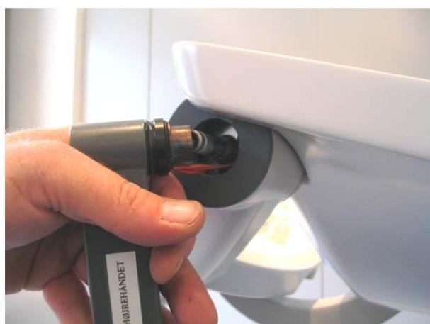
16. Tighten the hexagonal screw to obtain a suitable tension and friction for the arm movements.
