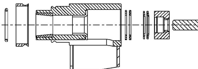
25. Exploded view orientation of the inside washers & spring-washers
