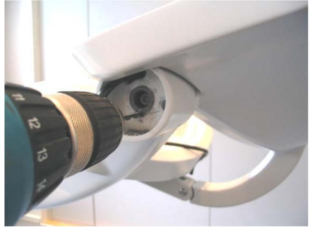
8. Cut M4 thread in the 3 holes. Use a small amount of cutting oil if necessary.
