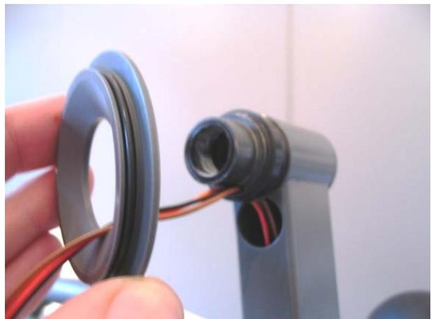
12. Pull the 4 wires from the suction hose holder out through the hole. Make sure the wires take up as little space as possible to leave room for the air hose of the lumbar support, if present.
