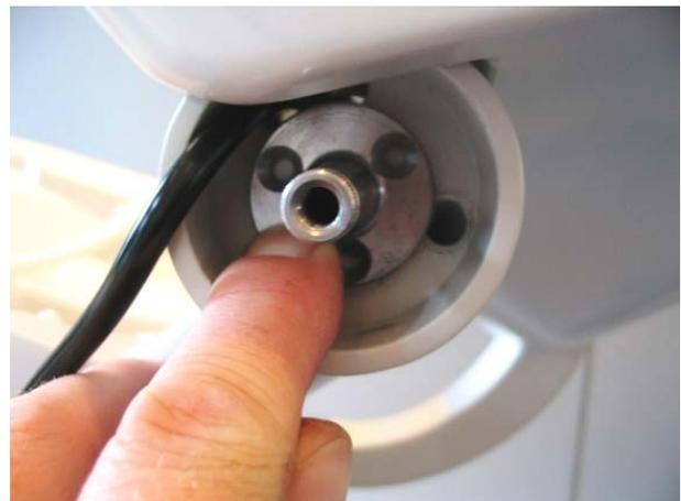
7. Drill the 3 holes using an  $\varnothing 3.3$  mm drill to a depth of min. 15 mm. It may be a good idea to drill one hole, cut the thread and fit the first screw. Then drill the other 2 holes, whilst the spindle is held in the correct position.
