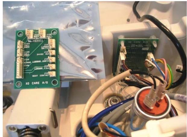
21. Wires and air hose fitted to cable holder with cable binders.
