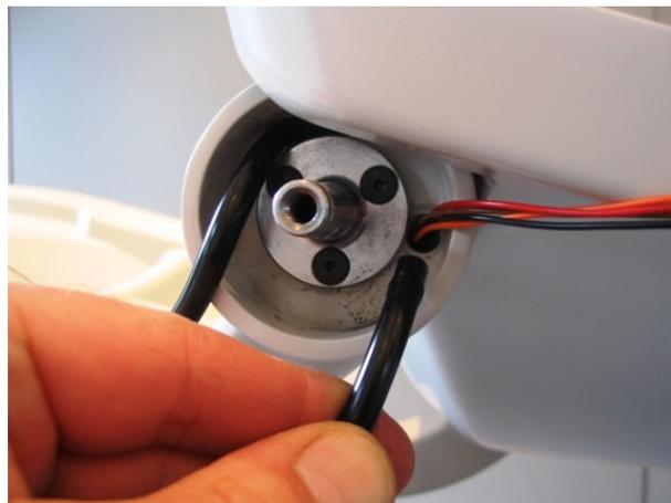
14. Carefully pull the wires (and air hose) through the hole until the suction hose holder can be fitted on the spindle.
