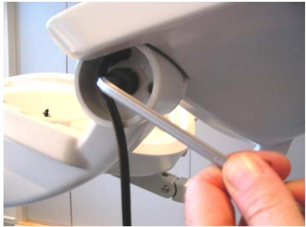
5. Pick the new MG-783 Threaded bushing from the kit and add Loctite 243 (UH-053) to the front part of the thread, before fitting.
