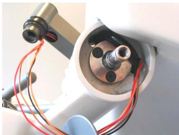
15. Fit the cover over the hole and press the arm onto the spindle.
