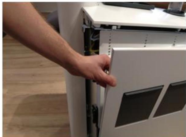
Place the filter bracket in the correct position.
