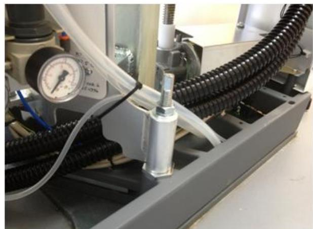
Measure the distance to the drain outlet in the floor. Cut the black drain hose in the correct length.
